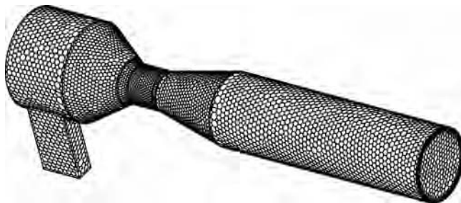
Figure 2.16. Polygonal surface mesh. Figure courtesy of M. Peric.
