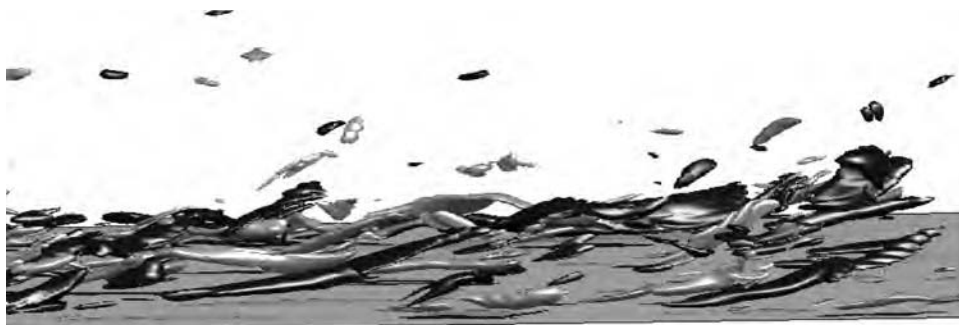
Figure 6.20. Isosurfaces of x vorticity near a wall in a perspective view. Dark gray surfaces are positive; light gray are negative.
