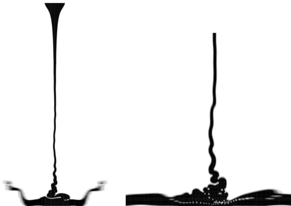
Figure 8.13. A stream of glycerine pouring onto a surface, computed with the volume of fluid method. Views at 1.45 and 1.5 s.
